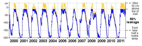
Left, an example from the updated model. The blue plot shows predicted water levels 2000-2011 with the existing weir height and 50% leakage. Reducing the leakage has increased the loss of water over the outlet, but much of this loss can be prevented by
