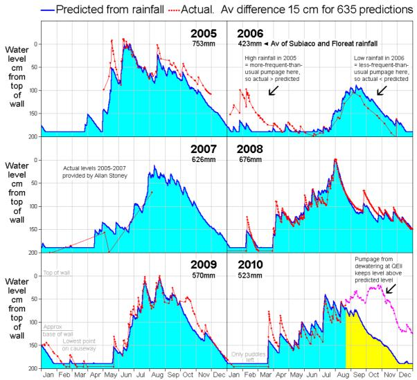
**Above,** the predicted levels (blue) closely match the observed levels (red), the average difference for 635 predictions during 2005-2010 being only 15 cm. And note how the days when the predicted level is at its highest is always close to those observed. But what happens if leakage is reduced? See next.
