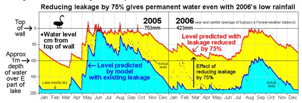
**Above,** even in 2006, permanent water could be achieved by reducing leakage to 25% of existing. Grey dots show the observed levels (repeated from the previous figure)
