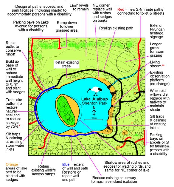
Main differences from SoJ proposals are: retaining only the wall shown in blue, realigning path along northern edge, no tiered seating in NW corner, even more reeds and sedges.
